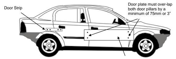
The Door plate must be fixed by either four 19mm bolts or studs, or six 13 mm bolts or studs, through both the door pillars. No slotted holes allowed
