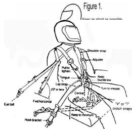
Fig.1 shows the location for the tail straps, which should be horizontal to 20<sup>0</sup> below horizontal, and as close to the shoulder as is practical for optimum restraint.
