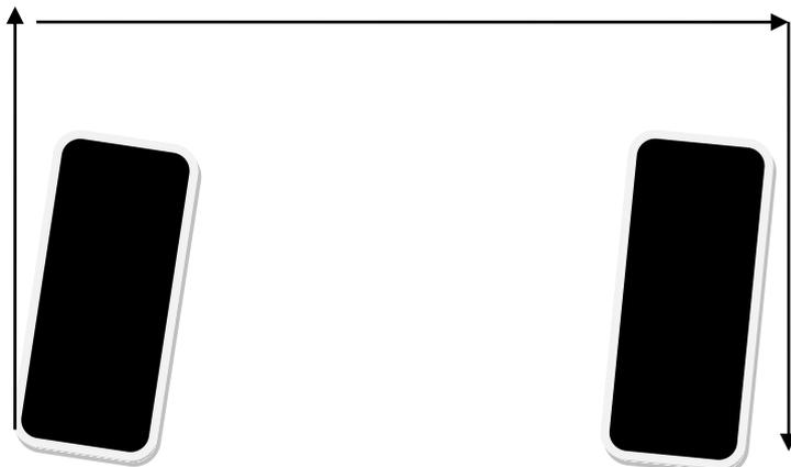
Front and rear track will include tyre and camber and castor and will be measured as shown not to exceed 55 1/4" overall width.
