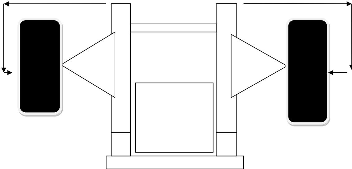
Rear End - top view looking down. Offset not to exceed ½” or 12.5 mm measured from outer chassis rails on both sides of car to inner lip of wheel as below.
