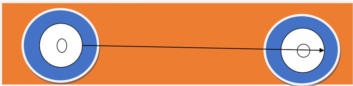
Wheelbase to be measured from either front of rim to back of rim in either direction not to exceed 76.5" or be below 76"
