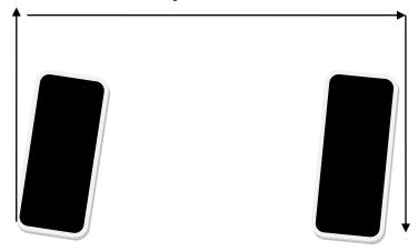
Wheelbase measurement points 59.5" (1511.3 mm) - 60.5" (1536.7 mm)
