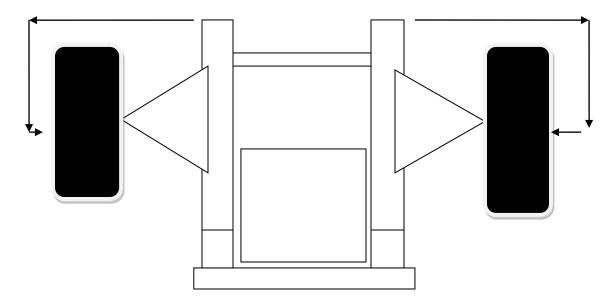
Rear end tech off set measurement points 0" - 1/2" or 0mm-12.7mm
